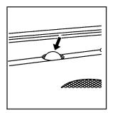
There is a solar sensor located on top of the instrument panel, near the windshield.
